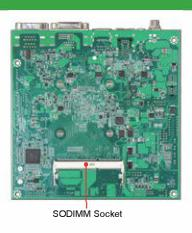
WADE-8079 is based on Intel® Atom™ processor E3800 product family with memory and PCI Express controller integrated to support two-channel DDR3L memory and PCI Express 2.0 lanes. Portwell has taken advantage of such technology to furnish a series of products that meets multiple industrial requirements for cost effectiveness, reliable performance and a high level of data integrity and uptime.
